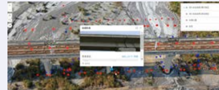
Inspection data is integrated with three-dimensional information of the bridge to perform detailed comparisons with historical photos.
