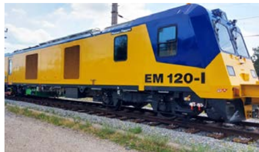
2024 Maintenance - track alignment inspection, track optical inspection
