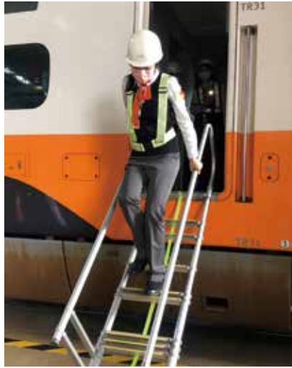
Train crew sets up escape ladder and conducts stability testing
